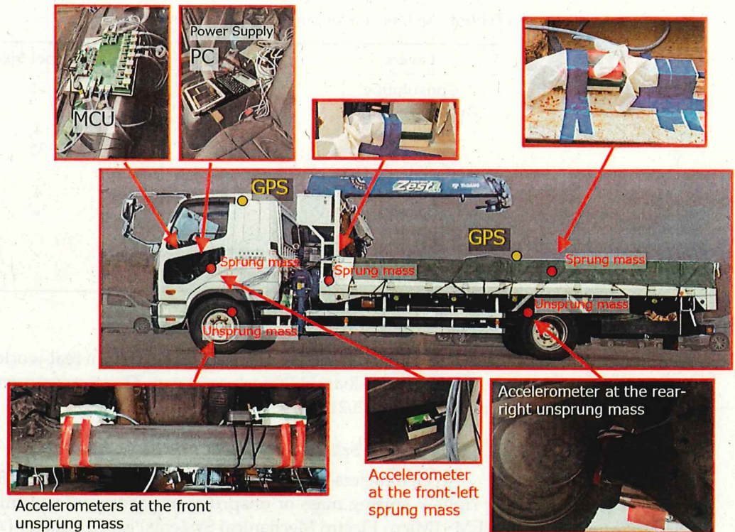
Figure 1. Vehicle and Accelerometers installation point.
